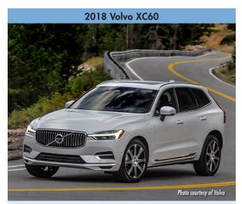
Type: Plug-in hybrid; SUV/Crossover EPA electric range: 18 miles EPA total range (gas + electric): 370 miles Charging time: 3 hours @ 240V; 6 to 9 hours @ 120V
