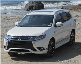
Type: Plug-in hybrid; SUV/Crossover EPA electric range: 22 miles EPA total range (gas + electric): 310 miles Charging time: 3.5 hours @ 240V; 8 hours @ 120V; Fast-charging capable
