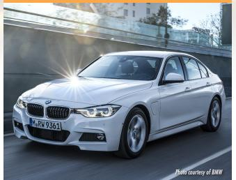
Type: Plug-in hybrid; Sedan EPA electric range: 14 miles EPA total range (gas + electric): 350 miles Charging time: 2.2 hours @ 240V; 7 hours @120V
