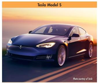
**Type:** Battery electric vehicle; Sedan **EPA electric range:** 335 miles **Charging time:** 4.75 to 8.75 hours @ 240V; Fast-charging capable
