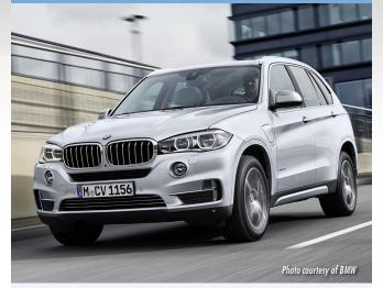
Type: Plug-in hybrid; SUV/Crossover EPA electric range: 14 miles EPA total range (gas + electric): 540 miles Charging time: 3 hours @ 240V; 6 hours @120V
