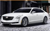
Type: Plug-in hybrid; Sedan EPA electric range: 31 miles EPA total range (gas + electric): 430 miles Charging time: 4.5 hours @ 240V; 10 to 15 hours @ 120V
