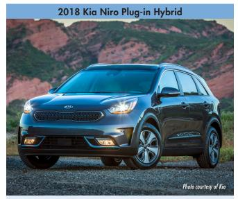
Type: Plug-in hybrid; SUV/Crossover EPA electric range: 26 miles EPA total range (gas + electric): 560 miles Charging time: 2.5 hours @ 240V; <9 hours @ 120V
