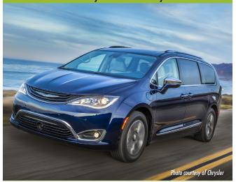
Type: Plug-in hybrid; Minivan/Wagon/Van EPA electric range: 33 miles EPA total range (gas + electric): 570 miles Charging time: 2 hours @ 240V; 14 hours @ 120V
