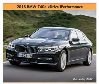
Type: Plug-in hybrid; Sedan EPA electric range: 14 miles EPA total range (gas + electric): 340 miles Charging time: 3 hours @ 240V; 7 hours @120V
