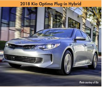
Type: Plug-in hybrid; Sedan EPA electric range: 29 miles EPA total range (gas + electric): 610 miles Charging time: 2.7 hours @ 240V; 9 hours @ 120V
