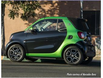
**Type:** Battery electric vehicle; Subcompact **EPA electric range:** 58 miles **Charging time:** 3 hours @ 240V; 16.5 @ 120V
