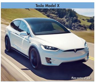
**Type:** Battery electric vehicle; SUV/Crossover **EPA electric range:** 295 miles **Charging time:** 6.5 to 9.5 hours @ 240V; Fast-charging capable
