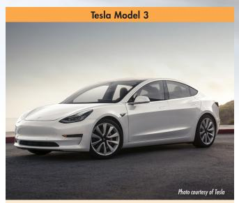
Type: Battery electric vehicle; Sedan EPA electric range: 220 to 310 miles Charging time: 8.5 to 12 hours @ 240V; Fast-charging capable
