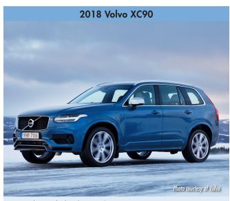
Type: Plug-in hybrid; SUV/Crossover EPA electric range: 19 miles EPA total range: 380 miles Charging time: 3 hours @ 240V; 6 to 9 hours @ 120V
