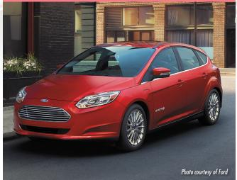
**Type:** Battery electric vehicle; Compact/Hatchback **EPA electric range:** 115 miles **Charging time:** 5.5 hours @ 240V; Fast-charging capable
