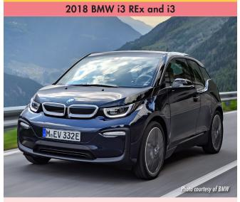
Type: Plug-in hybrid (i3 REx); Battery electric vehicle (i3); Compact/Hatchback EPA electric range: 97 miles (i3 REx); 114 miles (i3) EPA total range (gas + electric): 180 miles (i3 REx) Charging time: 5 hours @ 240V; Fast-charging capable
