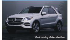
Type: Plug-in hybrid; SUV/Crossover EPA electric range: 10 miles EPA total range (gas + electric): 460 miles Charging time: 2 hours @ 240V; 7.5 hours @ 120V
