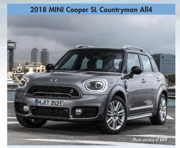
Type: Plug-in hybrid; SUV/Crossover EPA electric range: 12 miles EPA total range (gas + electric): 270 miles Charging time: 2 hours @ 240V; 4 to 6 hours @ 120V
