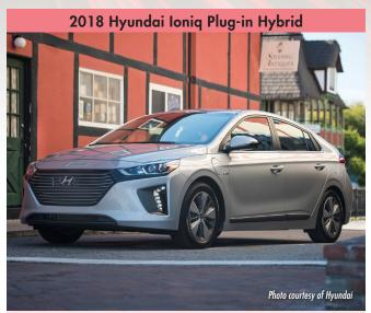
Type: Plug-in hybrid; Compact/Hatchback EPA electric range: 29 miles EPA total range (gas + electric): 630 miles Charging time: 2.3 hours @ 240V; 10 to 14 hours @ 120V
