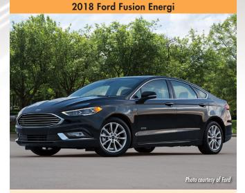
Type: Plug-in hybrid; Sedan EPA electric range: 21 miles EPA total range (gas + electric): 610 miles Charging time: 2.5 hours @ 240V; 7 hours @ 120V
