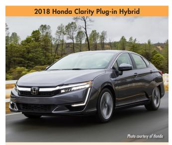
Type: Plug-in hybrid; Sedan EPA electric range: 48 miles EPA total range (gas + electric): 340 miles Charging time: 2.2 hours @ 240V; 16 to 24 hours @ 120V
