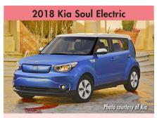
Type: Battery electric vehicle; Compact/Hatchback EPA electric range: 111 miles Charging time: 5 hours @ 240V; Fast-charging capable
