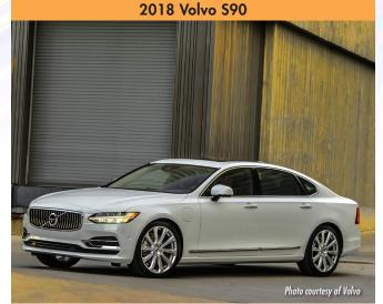
Type: Plug-in hybrid; Sedan EPA electric range: 21 miles EPA total range (gas + electric): 410 miles Charging time: 3 hours @ 240V; 7 to 10 hours @ 120V
